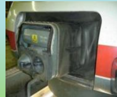
Protection of the coupler & local heating system
