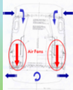
Roof air supply and installation of the body-shell under pressure
